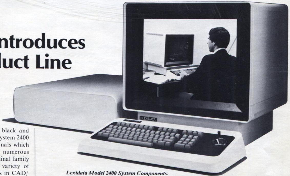
Lexidata Model 2400 System Components: Electronics Module, 19-inch monitor, and detachable keyboard with an integral joystick.
